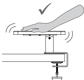
Prior to placing a device on the stand, push down on each assembled shelf to ensure stability.
