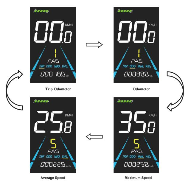
Figure 5-1 Display Interface Switching
