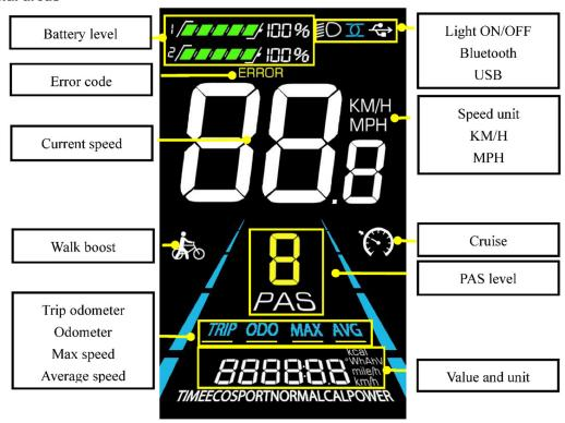
Figure 4-1 YL90T-V functional area distribution interface
