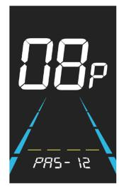
Figure 6-11 Pedal assist sensor magnets setting
