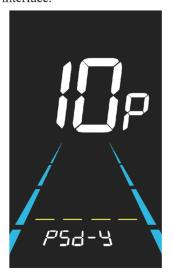
Figure 6-15 Password Activated interface
