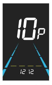
Figure 6-16 Power-on password setting interface
