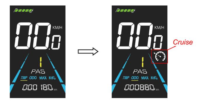
Twist the throttle for 8 seconds to achieve the fixed speed function
