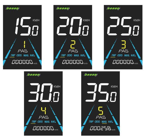
Figure 5-4 PAS level display interface
