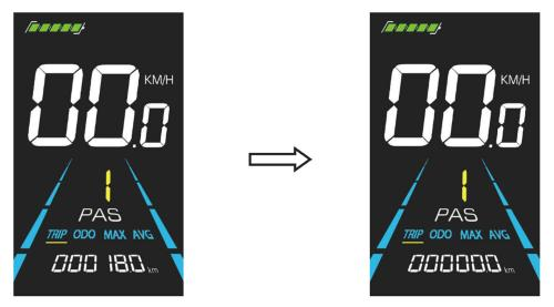
Figure 7-2 Trip Odometer Reset Interface
