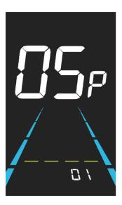
Figure 6-6 Number of speed sensor magnets setting interface
