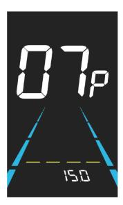
Figure 6-8 Controller current limit setting interface
