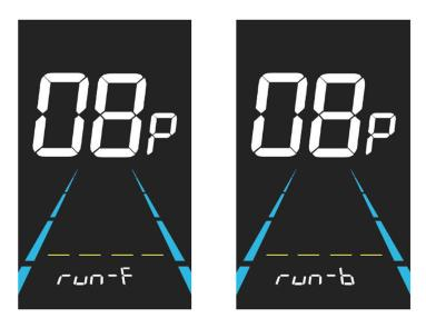
Figure 6-9 PAS sensor direction setting interface
