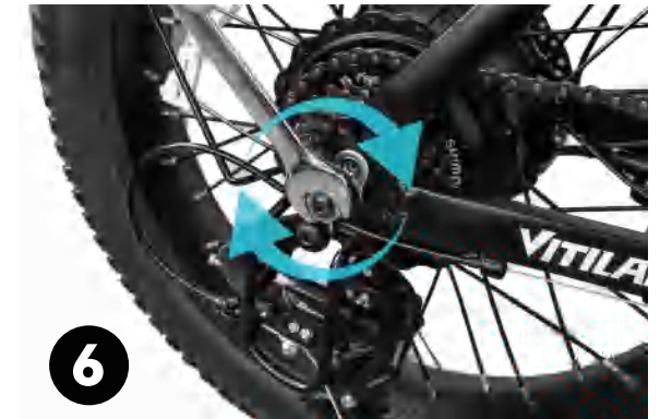
Step 6: Using an 18mm wrench to fasten bolt several times clockwise.
