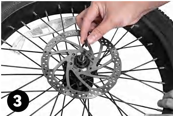
Step 3: Finding out 6 brake screws and put them into the brake mounting holes.
