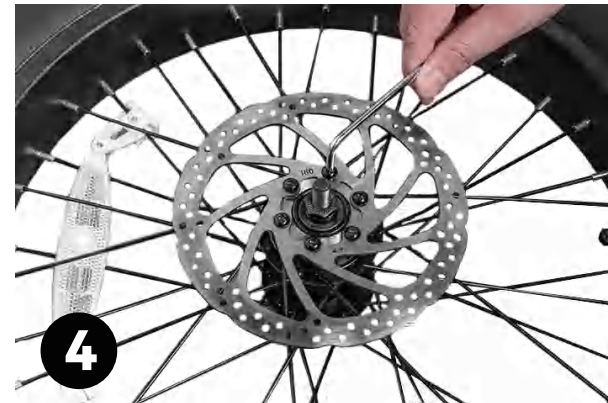
Step 4: Tightening the screws with a 4mm hexagonal tool.
