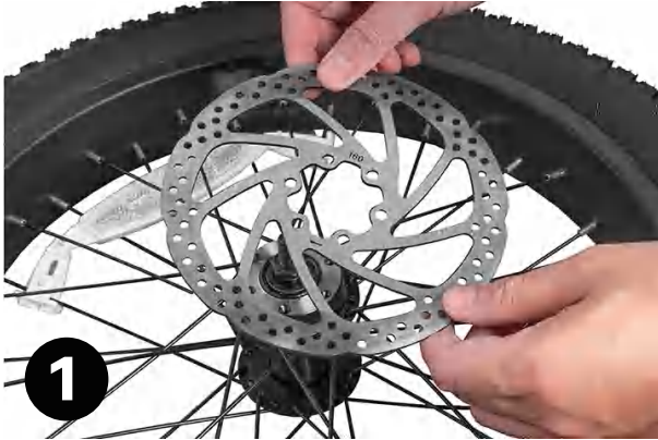
Step 1: Putting the brake rotor on the front wheel axle.
