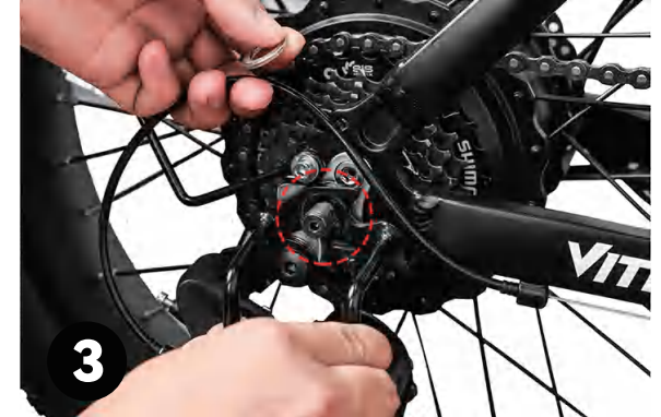
Step 3: putting the rear derailleur guard on the rear wheel axle.
