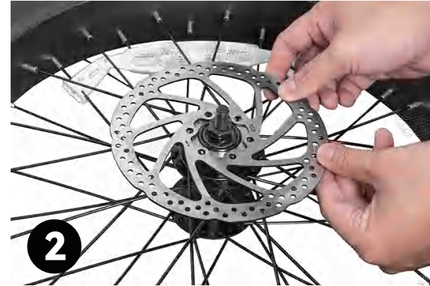
Step 2: Aligning the 6 holes on the brake rotor with the 6 corresponding holes on the axle.
