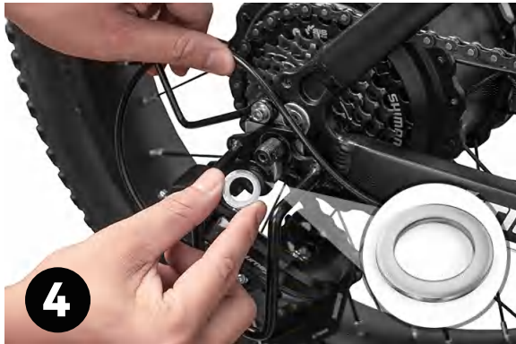
Step 4: Installing the spacer on the axle.
