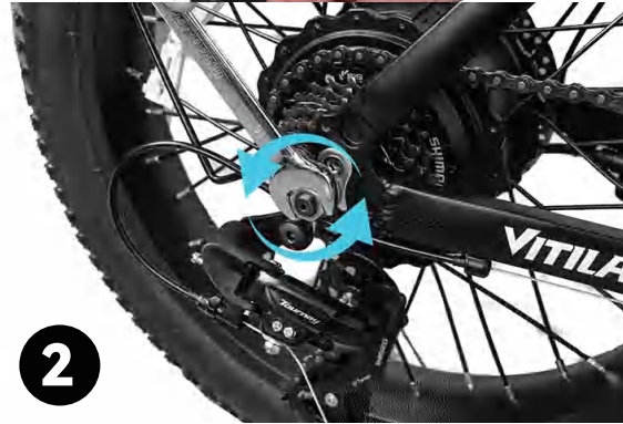
Step 2: Using an 18mm wrench to turn counterclockwise several times to loosen the bolt, loosen the spacer and bolt.
