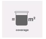
Coverage ≈ 3.4 kg/m² per 2 mm of thickness
