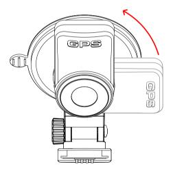
\*Adjust the GPS module counterclockwise to fix the bracket
