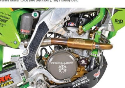
Surprisingly the engine is not highly modified. Besides the Rekluse clutch and JE Piston the internal components are OEM Kawasaki.
