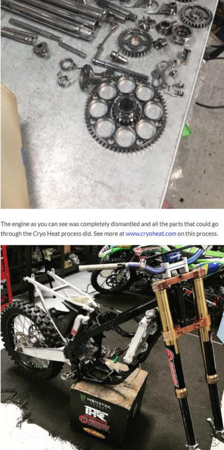
All the chassis bearings were replaced and treated as well. In person the black frame
