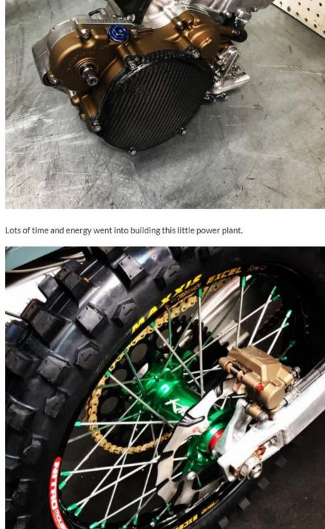
The wheel set is modernized using KITE hubs, Excel rims, Braking rotors, Renthal
