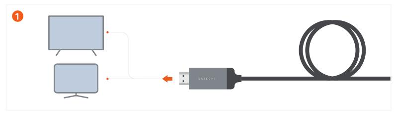
Connect USB-C to HDMI 2.18K cable into a compatible external display, monitor or television with available HDMI port. The Adapter is backwards compatible with HDMI 1.4 and up.
