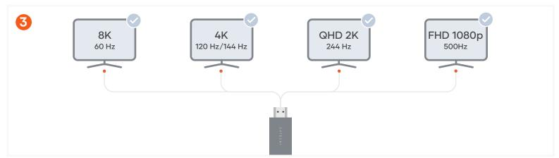
Cable supports the following outputs: 8K @ 60Hz, 4K @ 120Hz/144Hz, QHD 2K @244Hz, FHD 1080p @ 500Hz. Host device must support DP ALT Mode over USB-C.
