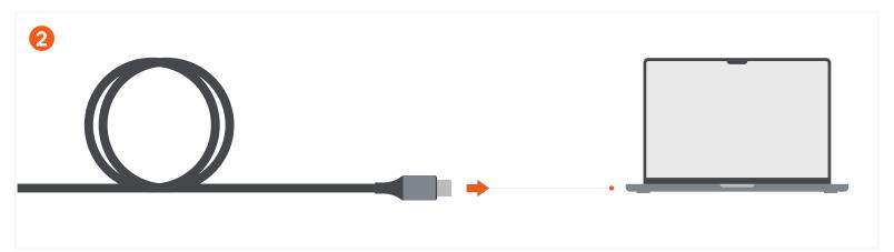
Connect USB-C to HDMI 2.18K Cable to your compatible host device.
