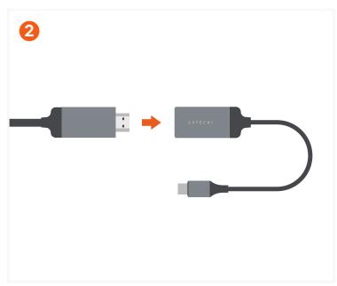
Connect second connector of an HDMI cable to the Adapter.
