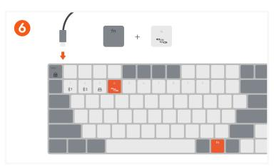
The keyboard can be used in wired mode by pressing "FN + 4" while the USB-C cable is connected to a host device port.
