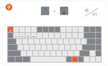
Press "FN + Esc" to activate the function key lock and swap between the Media and Function keys (F1-F12). Esc key will flash when function lock is enabled
