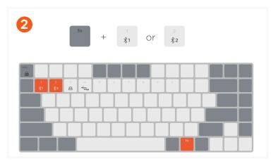
Press and hold FN key and one of the Bluetooth keys ("1" or "2") for ~5 seconds, until the LED starts to blink.
