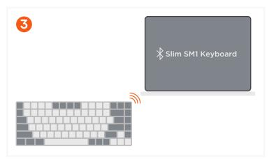
Select "Slim SM1 Keyboard" or "Bluetooth Device" on the host device's Bluetooth settings to complete the pairing process.
