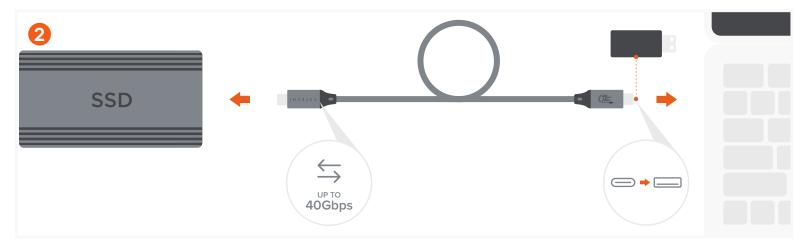
Connect USB4 cable to your USB-C or Thunderbolt 3/4 host devices for fast data transfer speeds up to 40Gbps. Backwards compatible with USB 3.2, USB 2.0 and Thunderbolt 3. USB-C to USB-A adapter not included.
