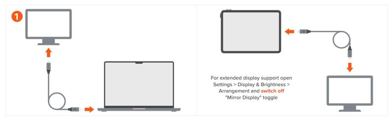
Connect USB4 Pro cable to USB-C or Thunderbolt external monitor. Supports single display 8K@60Hz or 4K@120Hz, and dual display 4K@60Hz. For dual display output must use two USB4 cables.
