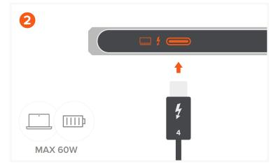
Using the included Thunderbolt 4 cable, connect the hub to your host device from its Thunderbolt 4 host port located at the front of the hub. Features 60W Max Pass-Through charging to the host device
