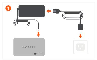
Connect the power adapter from the Hub's DC port directly to a wall outlet.
