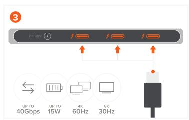
Connect up to three USB-C devices to the hub's Thunderbolt 4 ports. Supports up to 40Gbps & 15W charging. Supports dual 4K HDMI output up to 60Hz total or single 8K HDMI at 30Hz.
