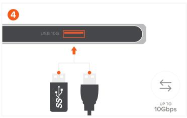
USB 3.2 Gen 2 port allows for transfer data at up to 10 Gbps speed.
