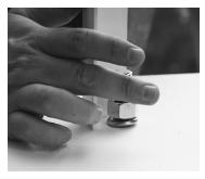
13. Tilting the column to one side may make it easier to position the rod so it can be inserted through the hole in the cap. Make sure that the attached angle is oriented properly. Caulk around the center hole. Only finger tighten the stainless steel nut at this time.
