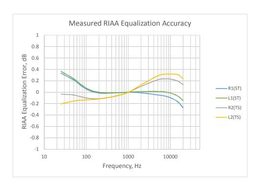
Fig. 4.1: Typical measured RIAA equalization error with both Sovtek 6H9C/6SL7GT (ST) and Tung Sol Reissue 6SL7GT (TS) tubes, left and right channels. Error is <0.5 dB from 25 Hz - 20 kHz for all curves.
