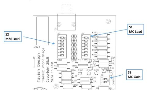
Fig. 3.2: Switch positions for setting MC Gain (S3), MM load (S2), and MC load (S1). For each switch, LEFT = OFF = 0, and RIGHT = ON = 1.
