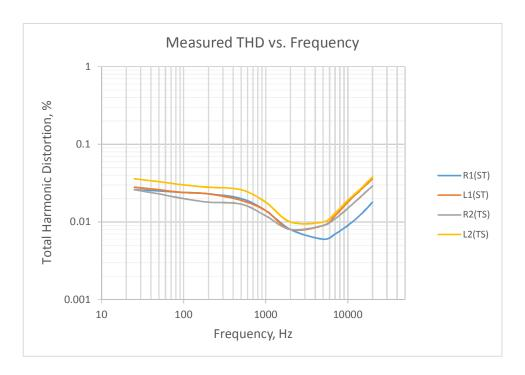
Fig. 4.2: Typical measured distortion over frequency, 560 mV RMS output level into 22 k $\Omega$ . ST = Sovtek 6H9C/6SL7GT, TS = Tung Sol Reissue 6SL7GT
