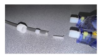
PUSH THE INSERT INTO THE CUT END OF THE TUBING SO THAT IT IS FULLY SEATED INTO THE TUBING.
