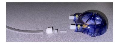
PUSH COMPRESSION NUT ONTO TUBING WITH THREADED END OF COMPRESSION NUT FACING CUT END OF TUBING.
