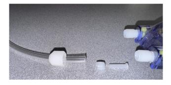
PUSH COMPRESSION RING ONTO TUBING, LEAVING A ½ INCH GAP BETWEEN THE COMPRESSION RING AND CUT END OF TUBING.
