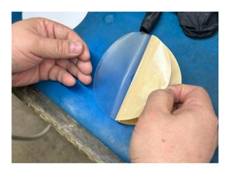
REMOVE WAX PAPER BACKING FROM DOUBLE-SIDED ADHESIVE AND AFFIX ONTO METAL BASE.
