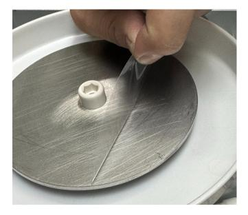
INSTALL NEW PLATEN TABLE RUBBER. FORM THE PLATEN TABLE RUBBER INTO A "U-SHAPE" AND PLACE HOLE OF PTR OVER CENTER PIN. STARTING IN THE CENTER AND WORKING TOWARD THE OUTER EDGE, USE YOUR FINGERS TO SET THE PTR TO THE ADHESIVE MAKING SURE TO REMOVE ALL AIR BUBBLES.
