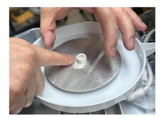
STARTING IN THE CENTER AND WORKING TOWARD THE OUTER EDGE, USE YOUR FINGERS TO SET THE ADHESIVE TO THE BASE MAKING SURE TO REMOVE ALL AIR BUBBLES. **REMOVE CLEAR COVERING FROM THE TOP OF THE ADHESIVE.** USING YOUR FINGERNAIL OR SHARP EDGE, REMOVE THE CLEAR TOP COVER OF THE DOUBLE-SIDED ADHESIVE.
