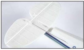
4. Place the elevator in position on the fuselage with the rudder pushrod above the elevator.
