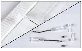
6. Install the aileron control horns to the ailerons in the same way as the elevator and rudder control horns. They should be on the bottom of the wing with the holes facing the servo. Then locate the bag with the 2 aileron pushrods and the aileron servo control arms shown in the photo to the left.
