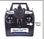
When the aileron stick is moved to the right of the transmitter the right aileron should move up and the left one move down. This will roll the wing to the right.
