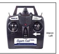
When the aileron stick is moved to the left of the transmitter the left aileron should move up and the right one move down. This will roll the wing to the left.
