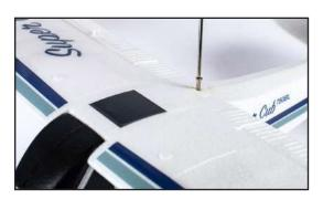
10. Place the wing in position on the top of the fuselage, making sure that the aileron servo wires are completely inside the fuselage, and screw into position with single screw (bag C) as shown to the left.
