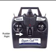
When the rudder stick is moved to the right of the transmitter the rudder should move right. When in flight this will yaw the tail to the left (the nose of the aircraft will move to the right).
