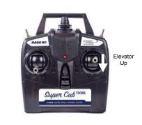
The PASS switch on the upper right of the transmitter should be in the OFF (toward back of transmitter) for these tests.
