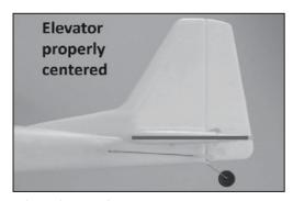
Then check that the elevator is properly centered as shown above.
