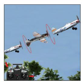
Press the Stunt Function Button then move the aileron stick in either direction to auto-roll the aircraft. After completing the roll the aircraft will return to level flight.
