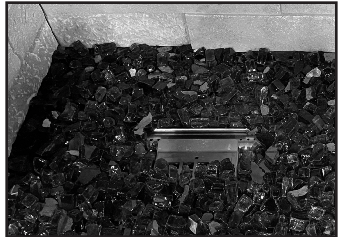
Figure 11.5 Media Placement Jig Removed
