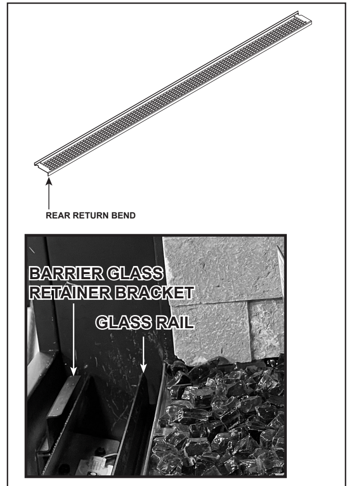
Figure 11.19 Install Transition Media Tray
