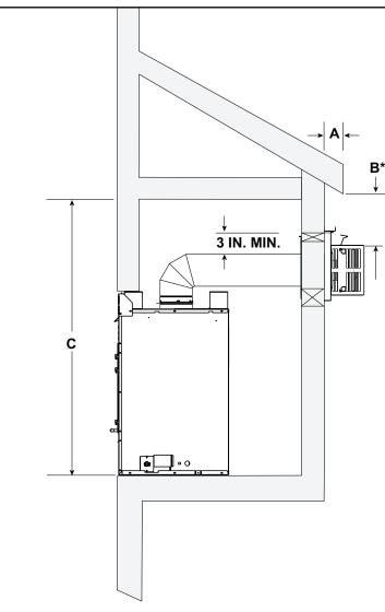
\* NOTE: If overhang is less than 2 inches, clearance from top of termination cap to bottom of overhang may be 0 inches.
