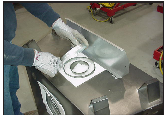
Figure 6.5 Remove the seal cap.
