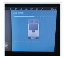
The machine will now run through a short 1 minute rinse cycle
