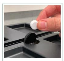
Drop a Franke cleaning tablet into the chute on top of the coffee machine and select NEXT
