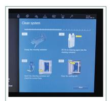
Once complete, empty the blue jug, fill with 50ml of cleaning solution and reinsert. Close door and select NEXT
