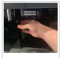
Open the door by removing the grounds container and pressing the red lever on the inside left of the door
