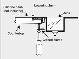
Note:Flush mount:Cut a groove precisely that can fit the top rim to ensure the sink top rim surface is level and flush with the coutertop surface
