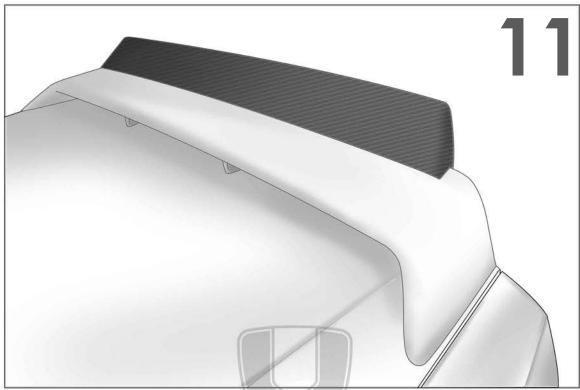
Once the urethane is cured, remove all of the tape holding the Crown in place as well as the tape at the bottom. Ensure that the Crown is well secured.
