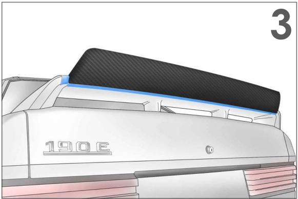
Place tape surrounding the entire Crown. This will prevent any excess urethane from contacting the paint.
