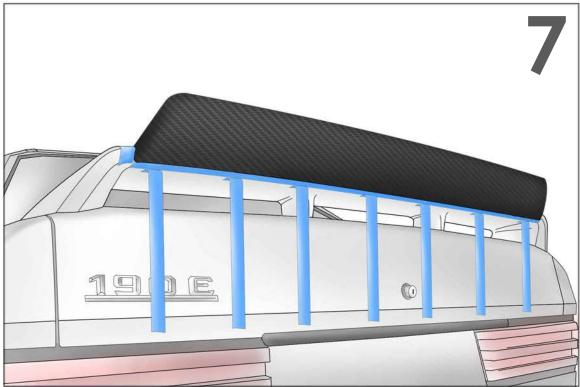
Carefully place the Crown onto the spoiler within the tape boundaries. Ensure that the angle is correct and that there is no gap on the sides.
