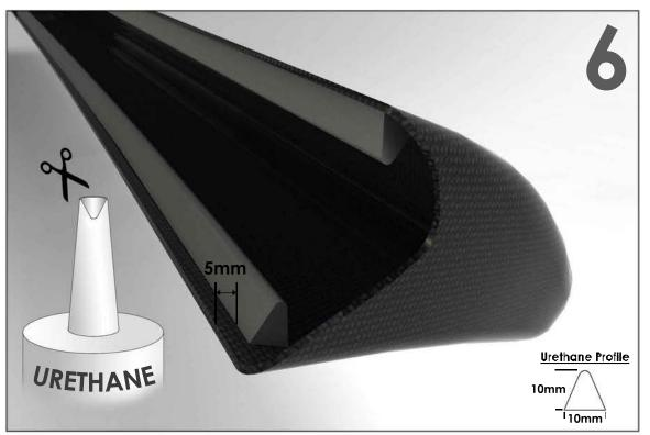
Lay a bead of windshield urethane, or similar, on each side of the inside of the Crown. Leave a 5 mm gap from the edge to the bead. The profile of the bead should be about 10mm X 10mm. Cut the urethane tube nozzle in a 'V' shape to get a pointed profile.
