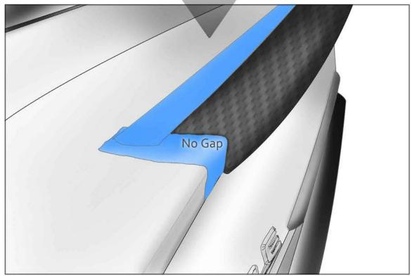
Adjust the angle until there is no gap on the sides where the Crown meets the spoiler.
