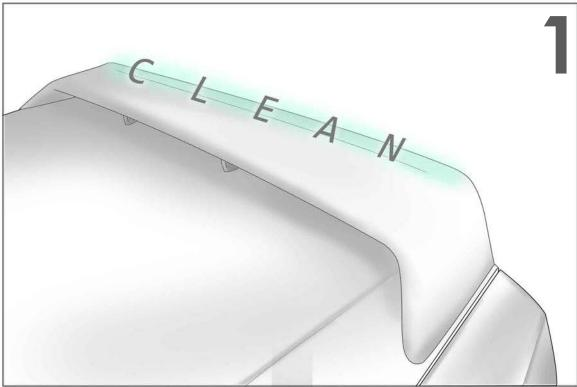
Thoroughly clean the area, that is shown in green, of the spoiler where the Crown will be mounted over. Use a wax and grease remover to sufficiently prepare the surface.
