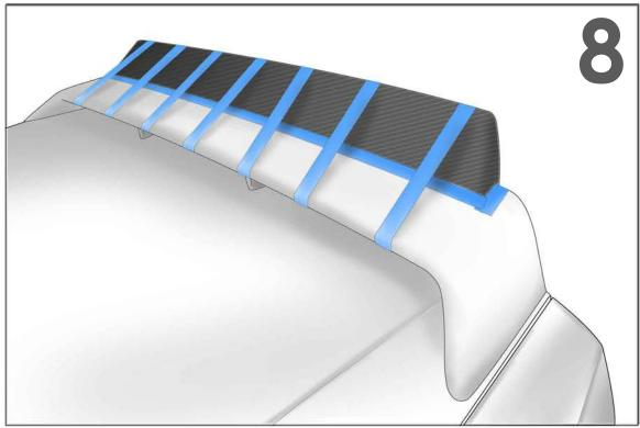
Wrap the tape firmly around the Crown and over the front edge of the spoiler.
