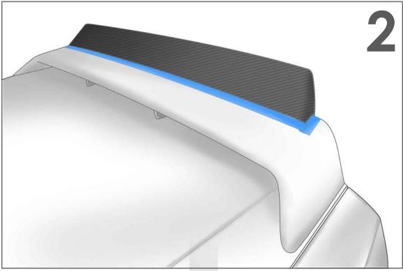
Place the Crown onto the spoiler ensuring that it is centered and at the correct angle for mounting. Stick painters tape on the spoiler up to the front edge of the Crown. (Use tape to temporarily hold the Crown in place if you are installing alone)
