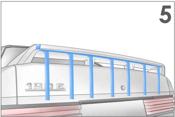
Measure out strips of tape approximately 18 inches in length. Stick them on the underside of the spoiler with the sticky side facing out. Place them around 5 inches apart.
