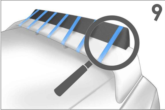
Remove the front and side pieces of tape. Inspect the Crown to ensure that it is well placed. If needed, secure with extra pieces of tape. Wipe off the excess urethane from the bottom piece of tape. (This tape will be removed later).
