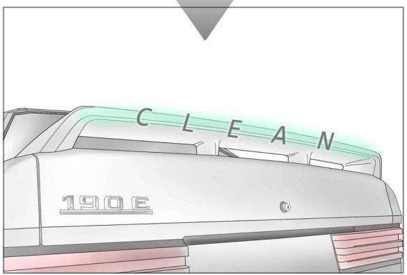
Ensure that you clean the back edge of the spoiler and underneath as well. Once wiped clean, let dry.
