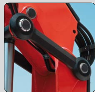
Forged double linkages on column and 2nd boom
