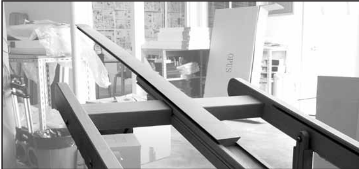
Figure 3d - Sliding the Mast Stem into place.
