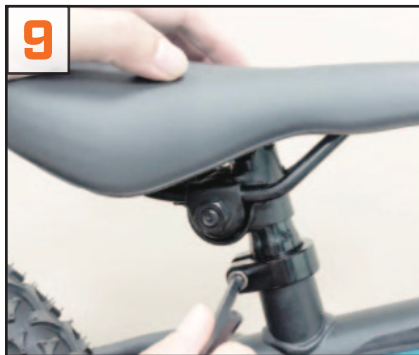
Loosen the seat clamp to adjust seat height. After adjustment, tighten the seat clamp using the 5mm Hex key.
