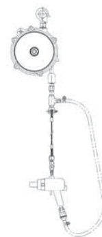
ATB-1 fitted with horizontal tool hanger
