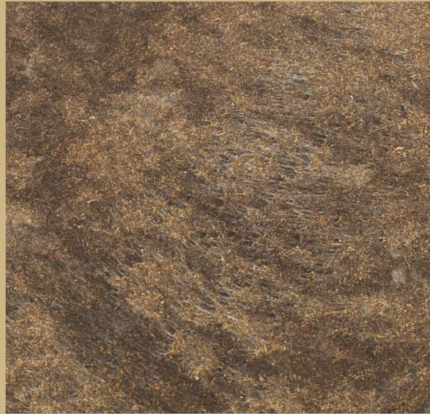
The Earth Stool seat is made from upcycled plastic waste from production of insulin pens mixed with beer fibre waste, thus creating a completely new innovative material finish.
