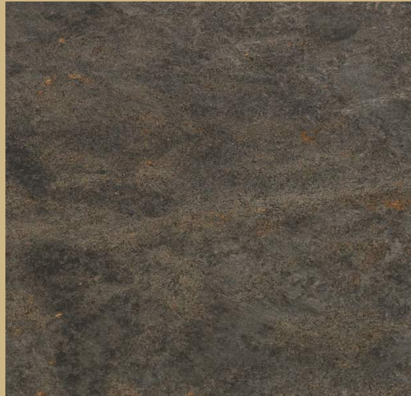
The Earth Stool seat is made from upcycled plastic waste from production of insulin pens mixed with coffee shell fibre waste, thus creating a completely new innovative material finish.
