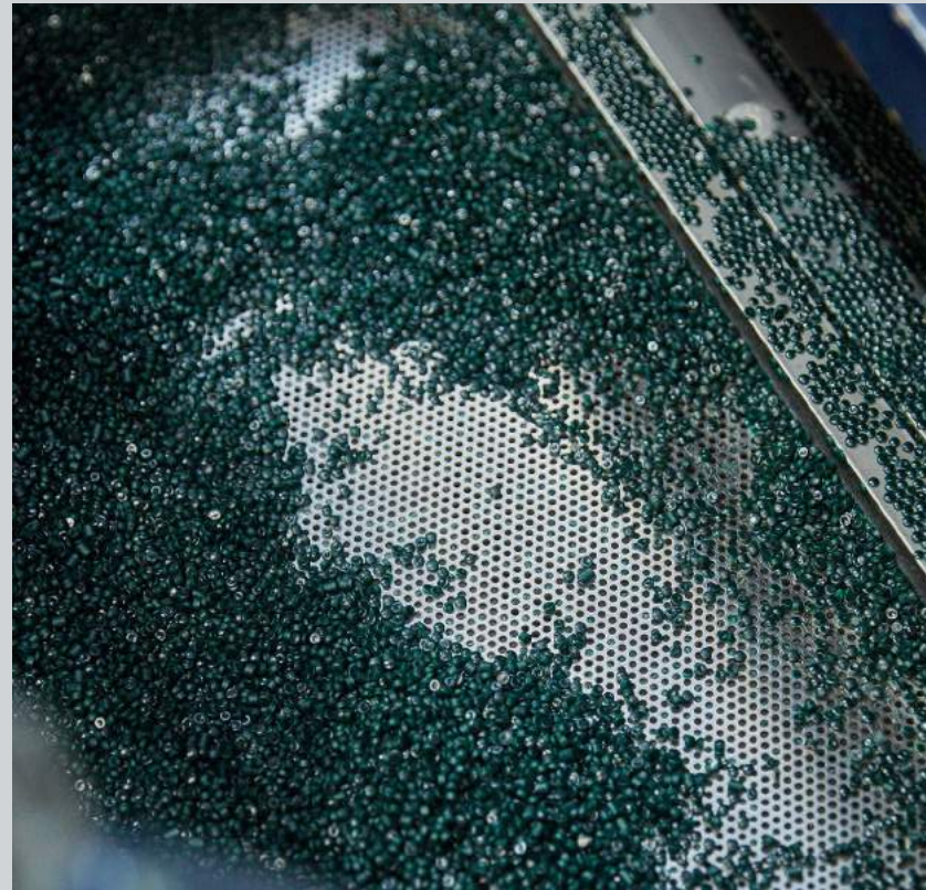
Discarded fishing nets made into green plastic pellets
