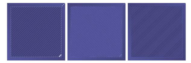
The following image illustrates the print direction of layer three when the **Skin Alternate Rotation** option is enabled.
