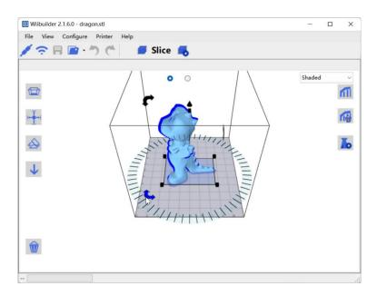
2. The model needs to be centered and correctly placed on the platform. Click "Center Object", "Flat", and "Land object".
