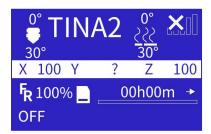
Info Screen displays the status of the main components, including: Nozzle temperature (preset temperature and actual temperature), heated bed temperature (preset temperature and actual temperature), network connection status, XYZ position information, remaining printing time, and TF card status.
