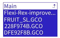
Select a file and press the knob. The next screen will show the printing information of the gcode file. Select "Print" will start printing. To prevent damage to the 3D printer, the system will check the machine model parameter in the gcode file. If the machine model parameter is not match or missing, the gcode file will not allowed to print. Please use the Wiibuilder or the customized version of Cura, select the correct model for slicing.
