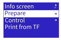
Press the knob to open the prepare menu. This menu has two screens, turn the knob to scroll the screen.
