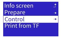
Press the knob to open the control menu. This menu has three screens, turn the knob to scroll the screen.
