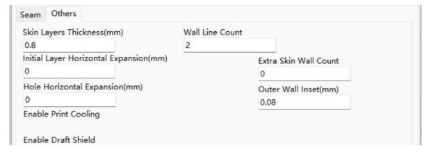
Skin Layers Thickness (mm): This option determines the thickness of the top and bottom skin layers.
