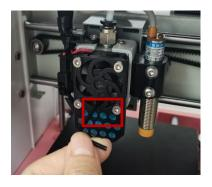
2. Open the buckle and remove the Hotend from the bottom. The disassembly process of the Hotend is complete.
