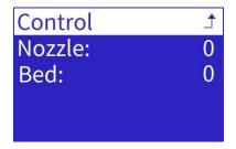
Turn the knob clockwise to reach the desired temperature, and press the knob to confirm. After the 3D printer starts to heat up, the home page will display the real time temperature of the nozzle.
