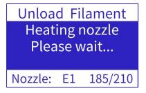
The nozzle will be heated to 210°C, then the extruder will retract the filament from the nozzle. During heating or extrusion, you can press the knob button to exit the current operation.
