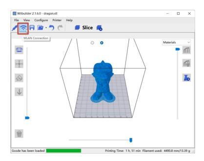
2. Click "WLAN Connection", the software will automatically search for the 3D printers in the local network and show them in the below list. If no 3D printer be found, you can also try to manually enter the IP address of the 3D printer to connect.
