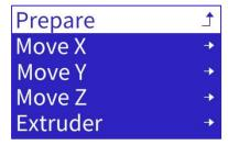
Click "Move axis", click the adjustment buttons of X, Y, Z, and control the movement of the X, Y, and Z motors respectively. The distances of X.Y.Z axis: 10mm, 1mm, 0.1mm respectively. The distance of the extruder motor: 10mm, 1mm, 0.1mm. In the debugging interface of each axis, the knob can control the bidirectional operation of the axis motor.
