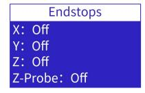
**Fault**: Click the X, Y, Z endstop by hand, and observe whether the interface status is changed. Use a metal object to approach the bottom of the Proximity Sensor, observe whether the interface status changes, and whether the light of the Proximity Sensor is on.
