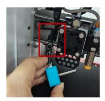
3. A new Hotend can be installed and replaced by operation in the reverse direction. After replacing the Hotend, the platform needs to be re-calibrated to start printing the model.
