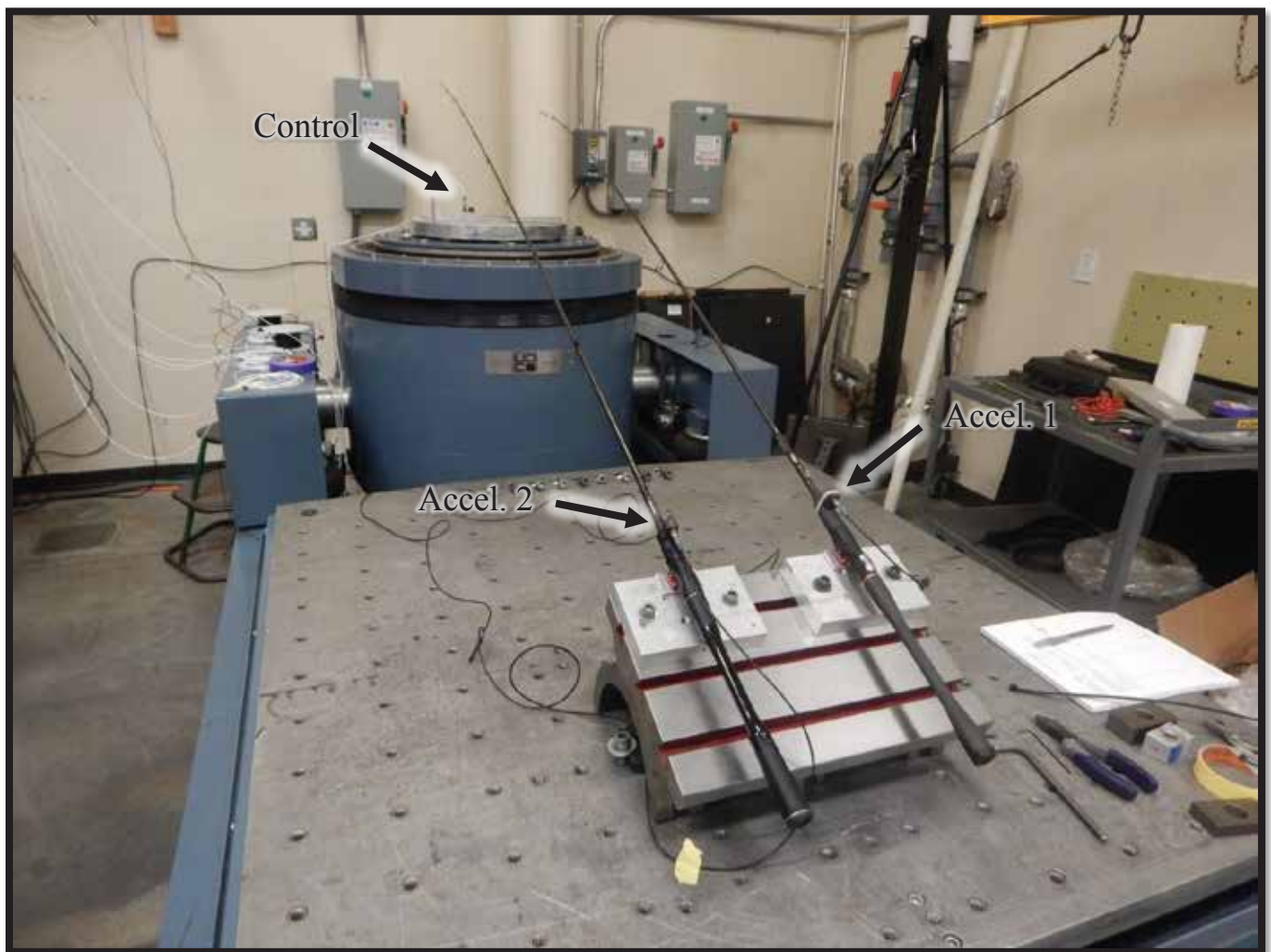
Figure 4-1: The test configuration for the spinning type rods. The accelerometers are indicated as Control, Accel. 1 (Channels 2 - 4) and Accel. 2 (Channels 5 - 7). Shown are the Trika rod on the right and the Competitor #2 on the left.
