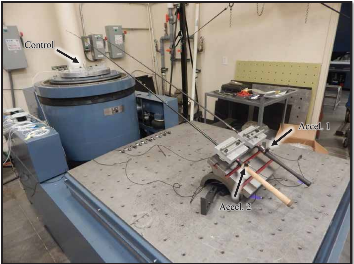
Figure 4-2: The test configuration for the casting type rods. The accelerometers are indicated as Control, Accel. 1 (Channels 2 - 4) and Accel. 2 (Channels 5 – 7). Shown are the Trika rod on the right and the Competitor #1 on the left.
