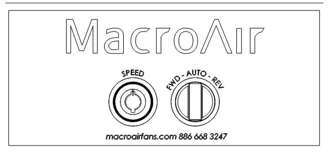
**OFF:** To turn off the fan set to FWD (forward) or REV (reverse) with a speed of 0. This will turn the fan off and prevent the BMS from running the fan.
