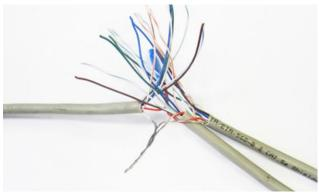
7. Repeat steps 3-5 for all the wires EXCEPT the Brown/White wire. The Brown/White wire is only needed for wiring in a repeater.
