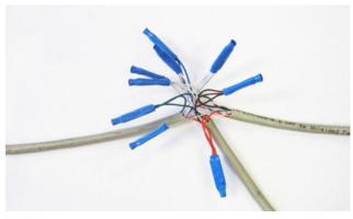
8. Once all the wires are crimped, carefully twist the wires up. Then fold them back and tape them up with electrical tape to clean up your wiring.
