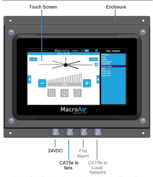
Note: The glands for the fire alarm and CAT5e to local network are plugged from the factory in order to maintain the screen's IP 66 rating when not used. If you are utilizing the fire alarm option and/or remote operation, remove the plugs from any gland you will be using.
