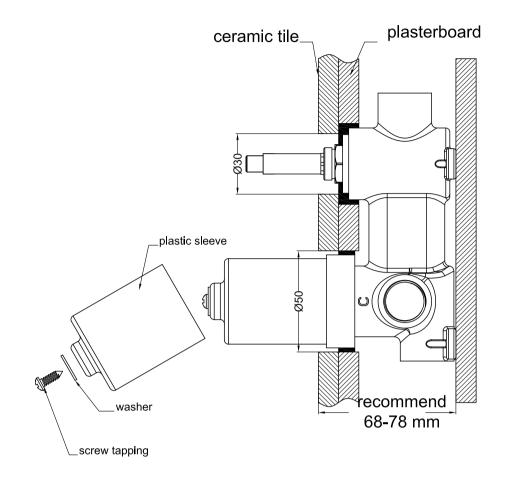
1.Drill a  $\phi 50$  and a  $\phi 30$  hole on ceramic tile, then install ceramic tile according to above picture.
