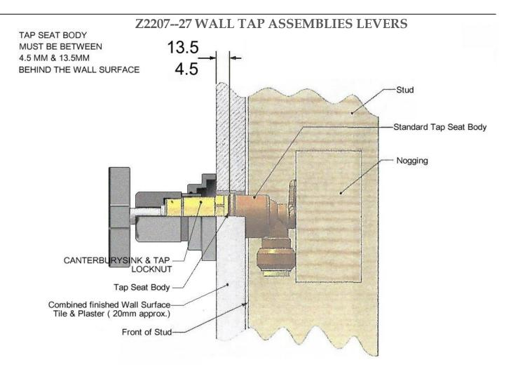
• A small amount of silicon can be applied behind the flange to hold it in place.
