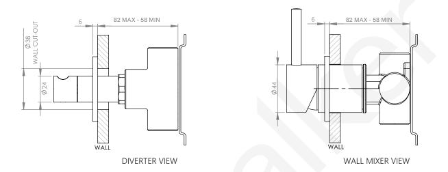
Ensure water lines are completely flushed prior to connecting the mixer.
