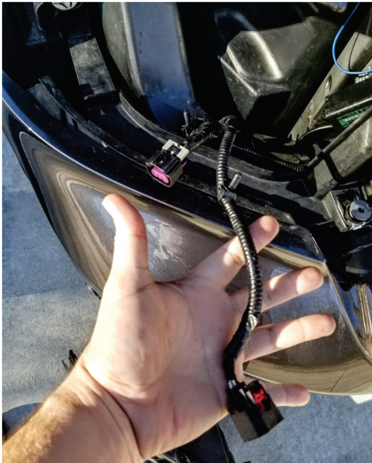
Connections from the truck - headlight plug on left, park / turn on the left.
