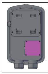
1- Loosen four screws of the input cable cover on the rear of the charging unit.
