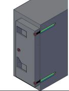
5- Ensure the screws are secured fully and the wall bracket is not loose.
