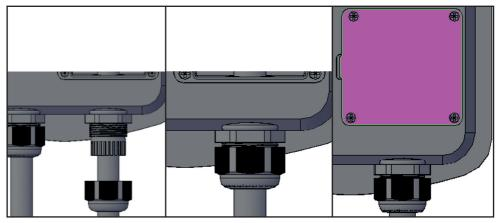
**7-** Install the rubber ring into the end of the gland along the cable.
