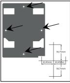
1- Wall bracket should be placed flat on the wall at an appropriate position, and the screw hole position shall be marked (or marked in mm according to the above figure).
