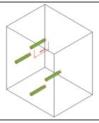
3- Insert the rubber plugs, ensuring the surface of the rubber plug is flush with the wall surface.
