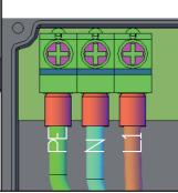
**6**- The input cable passes through the gland nut and rubber ring in sequence. Then go through the inner hole of the cable gland and enter the wiring sequence from left to right, PE, N, L1. Terminals must be tightened securely.
