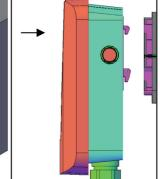
6- Attach the charging unit to the wall mounted bracket by matching the clips and sliding it down.
