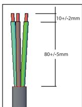
4- Use a 3-core 6mm<sup>2</sup> multi-strand flexible copper cable. See the figure above for the stripping method (it is better to crimp the terminal at the end of the cable).
