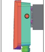
7- Push the unit towards the wall to check it is properly clipped on.
