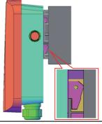
**8**- Push the unit downwards so **9**- Lock the anti-theft screws that it is completely clipped on. into the holes on both sides of
