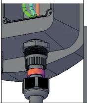
**5**- The input cable passes through the gland nut and rubber ring in sequence. Then pass through the inner hole of the gland and enter the inside of the charging unit.
