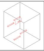
2- Use a 6mm drill bit to drill holes at the marked position, with the depth>40mm.
