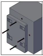
4- Secure the wall bracket to the wall ensuring it is the correct way up (as shown in the diagram).
