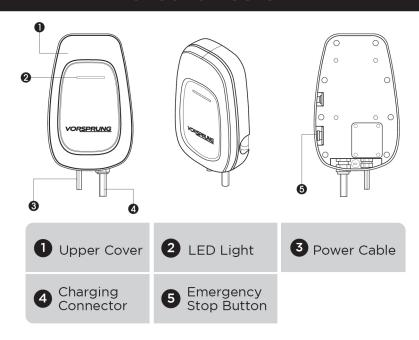
**NOTE:** Do not use the emergency stop button as a stop switch, if the emergency stop button is pressed, please reset it by twisting the button clockwise.
