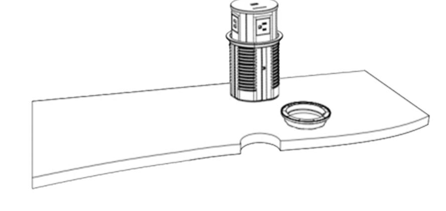
3) Replace the lock ring and turn it to secure the socket in place.
