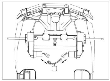
As shown in the figure: Connect the motor wires.
