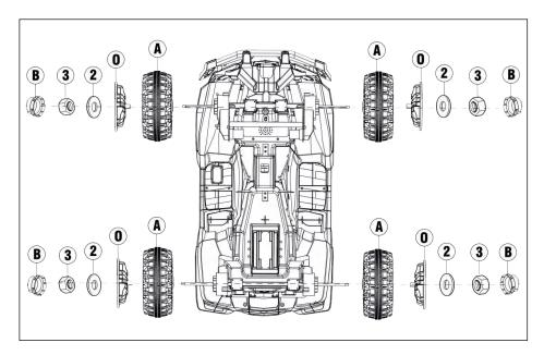
Put the wheel, wheel hub, gasket and nut into the front axle in turn.
