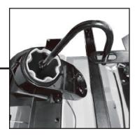
W Insert the steering lever into the steering motor hole.
