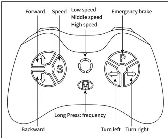
**Remote control first. When the remote control is on, foot pedal is not workable.**
