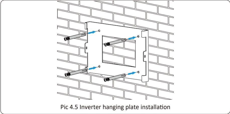
2. Ensure that the position of the installation holes on the wall is in accordance with the mounting plate, and the mounting rack is vertically placed.
