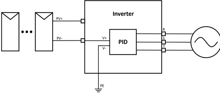
The Anti-PID module repairs the PID effect of the PV module at night. The PID module always runs when connected to AC. If maintenance is required and turn off the AC switch can disable the Anti-PID function.
