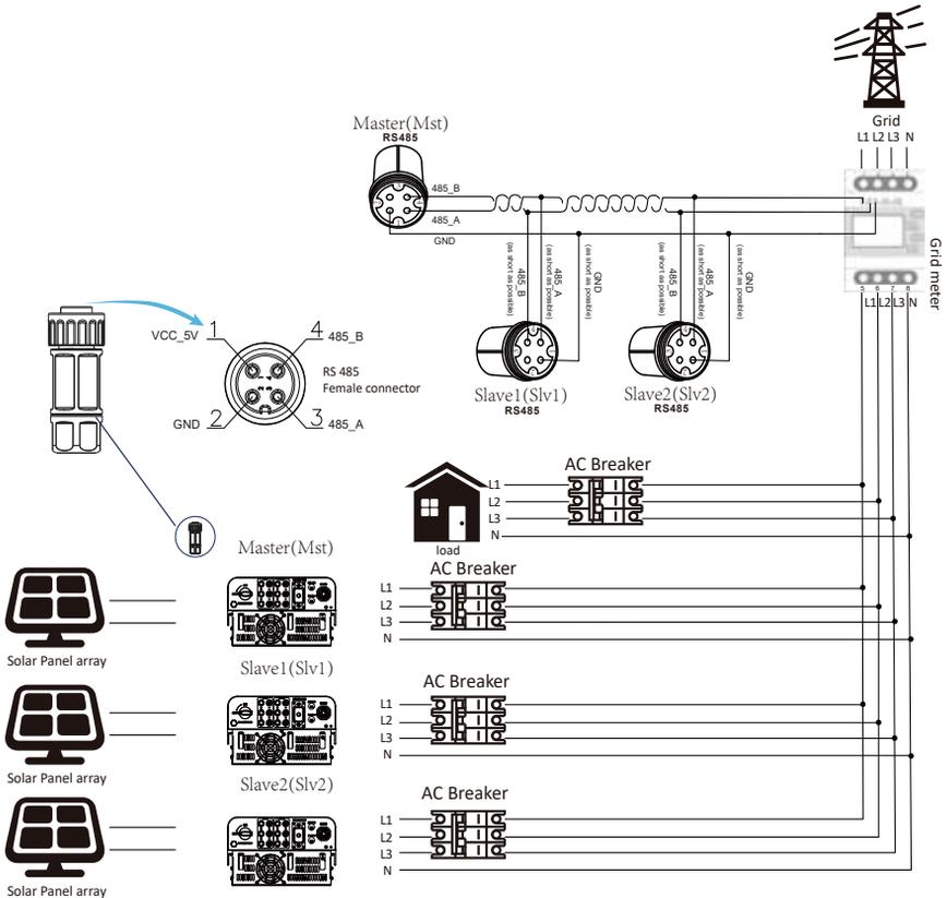
Pic 7.11 Eastron Connection diagram(The pass-through table)
