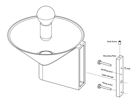
Outdoors: This light can be installed outdoors if installed in the downward facing position. In this application, it is best to wire it low voltage 12/24V.
