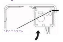
Hook the back of the headrail into the bracket and rotate the headrail into position. Secure headrail by tightening the short screw in the front of the bracket.
