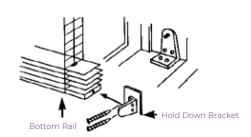
Hold down brackets: Using two small screws, screw hold down bracket to window facing or wall. Snap bracket pin ends into the hole at bottom rail end caps.
