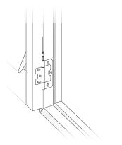
To mount the doors, hold the door in place then line up the prefitted hinges on the door and the frame. Once you have done this, slide the hinge pin vertically through the hinges to lock them in place.
