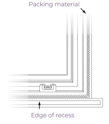
Lift the frame into the recess in the position you wish to fix it. Make sure the frame is level, using shims or packers and a spirit level, and ensure the frame is fitted squarely into the recess. Use a tape measure to centre the frame.
