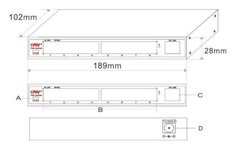
A. Multi-function Switch (S: Standard Setting, E:10M/250 Meters, V:VLAN)
